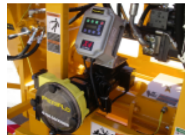
Chemical additives pump
